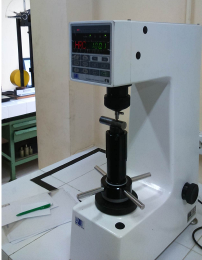
Gambar 2.3 Hardness Rockwell Digital
